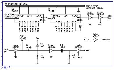
LD on the 74HC165's HIGH. This will load the data at their serial input pins (Only two of five IC's are shown). Inverter 1/4A supplies the clocking for the HC165's so that on each falling edge of the PSX's supplied CLK the next bit of data in the HC165's is shifted out. This data out is gated by the ATT signal on inverter 2/4B, this is so only the selected device can drive the bus.
