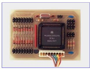
The micro controller version uses the Motorola 68HC11 (no one presented a compelling argument to use anything different). The code is currently set up to assemble for an E2 but can be changed to run on any 52 pin version with EEPROM (I made sure that I didn't use interrupts or use more than 256 bytes).
