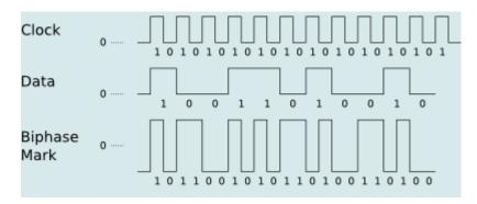
The frequency of the clock if twice the bitrate. Every bit of the original data is represented as two logical states, which, together, form a cell. The length of a cel ('time-slot') is equal to the length of a databit. The logical level at the start of a bit is always inverted to the level at the end of the previous bit. The level at the end of a bit is equal (a 0 transmitted) or inverted (a 1 transmitted) to the start of that bit.
