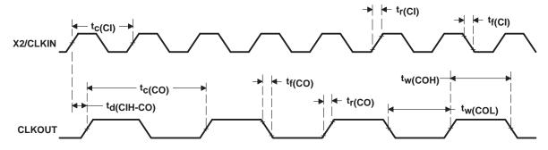
Figure 11. External Divide-by-Two Clock Timing
