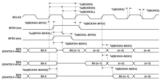
Figure 29. McBSP Transmit Timings
