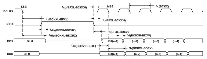
Figure 31. McBSP Timing as SPI Master or Slave: CLKSTP = 10b, CLKXP = 0
