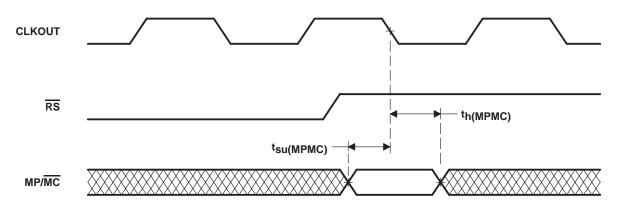
Figure 24. MP/MC Timing
