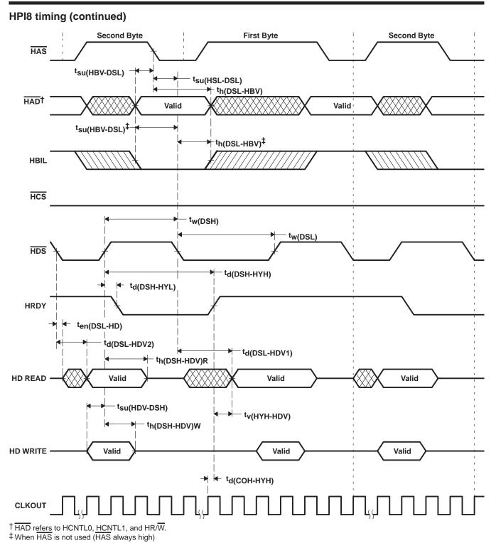
Figure 35. Using HDS to Control Accesses (HCS Always Low)
