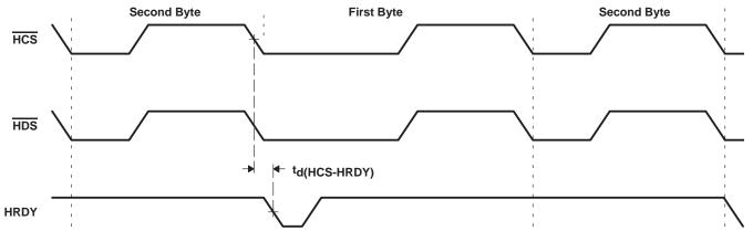
Figure 36. Using HCS to Control Accesses
