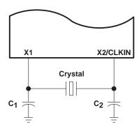
Figure 10. Internal Oscillator With External Crystal
