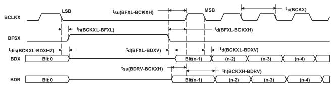
Figure 32. McBSP Timing as SPI Master or Slave: CLKSTP = 11b, CLKXP = 0
