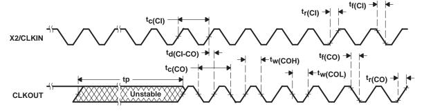
Figure 12. External Multiply-by-One Clock Timing
