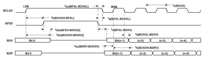
Figure 33. McBSP Timing as SPI Master or Slave: CLKSTP = 10b, CLKXP = 1
