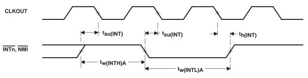
Figure 23. Interrupt Timing
