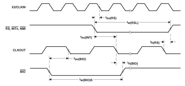
Figure 22. Reset and BIO Timings
