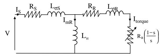
Figure 5: Steady State Phase Electrical Model
