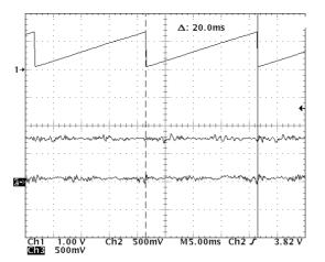
Figure 18: Rotor Flux Position, Flux and Torque Components
