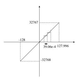
Figure 11: 8.8 Numerical Format Correspondence Diagram
