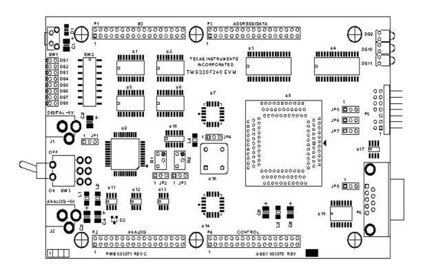
Figure 1: Top View of the TMS320F240 Evaluation Module
