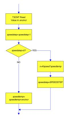
Figure 13: Speed Feedback Computation Flowchart
