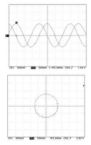
Figure 15: Output of the Clarke Transformation Module
