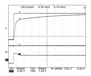
Figure 32: Speed Reversion from -1000rpm to 1000rpm under nominal load
