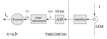
Figure 8: Current Sensing and Scaling Block Diagram
