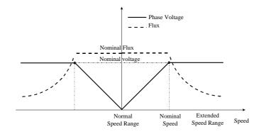
Figure 22: Field Weakening Voltage Constraints
