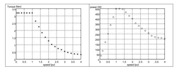
Figure 25: Experimental Torque & Power Charact. in the Extended Speed Range
