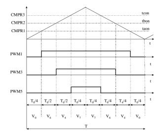
Figure 27: Sector 3 PWM Patterns and Duty Cycles
