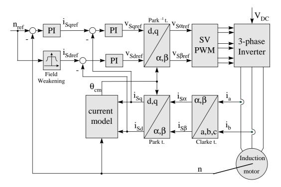
These two induction motor control dedicated modules are added to the basic FOC structure. This results in the following complete FOC AC induction drive structure:
