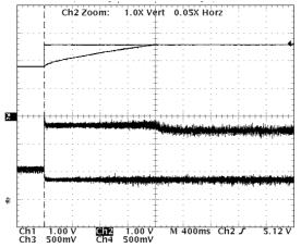
Figure 31: Transient Operation in the Extend. Speed Range / Torque Limit. set to 1
