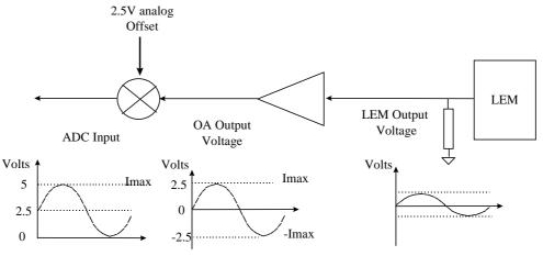
Figure 9: Current Sensing Interface Block Diagram
