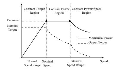
Figure 20: Field weakening Real Operation
