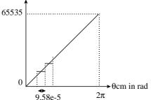
Figure 16: Link between Rotor Flux Position and its Numerical Representation
