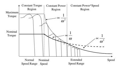
Figure 21: Maximum and Nominal Torque vs Speed
