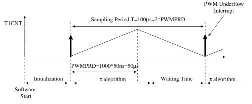
Figure 4: FOC Software Initialization and Operating System
