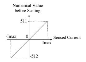
Figure 10: Sensed Current Values before Scaling
