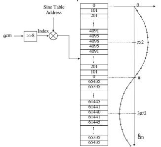
Figure 19:  $Sin\theta_{cm}$  Calculation using the Sine Look-up Table
