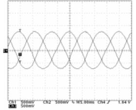
Figure 14: AC Induction Drive Phase Currents
