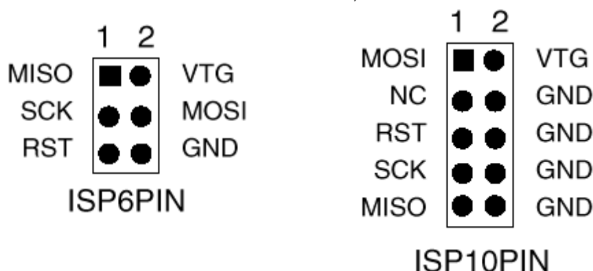
Figure 4-1. Standard ISP connectors on STK500, AVR ISP and STK200/STK300
