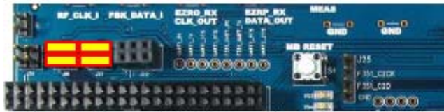
Figure 2. Jumper Positions (JP19, JP21)
