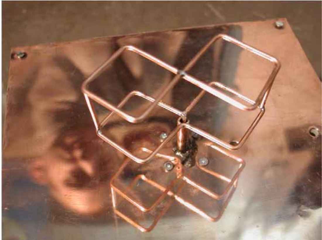
Fig. 21. Feeding of 2 el. bi-quad feed antenna 图. 21. 叠加双菱馈源天线的馈电
