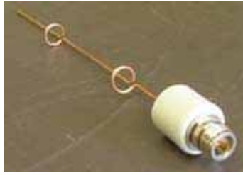
N-type connector screwed into an end cap
