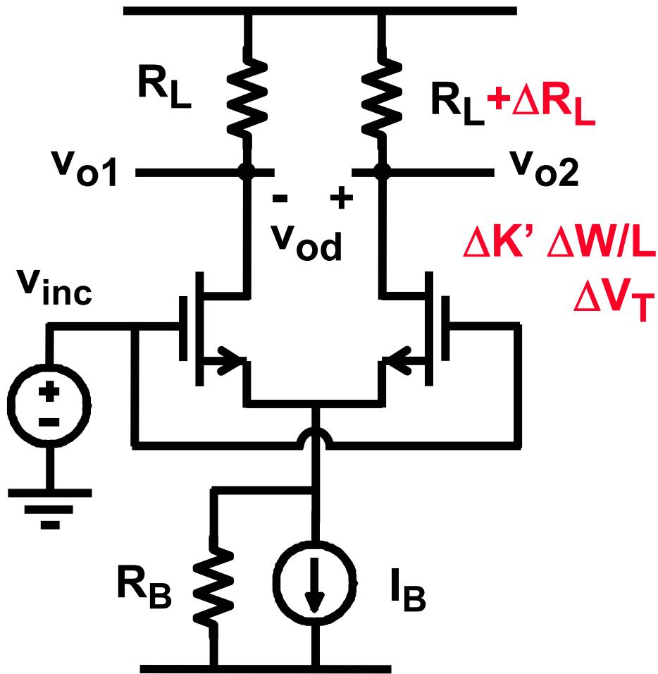
$$v_{od} = A_{dd} v_{id} + A_{dc} v_{ic}$$
