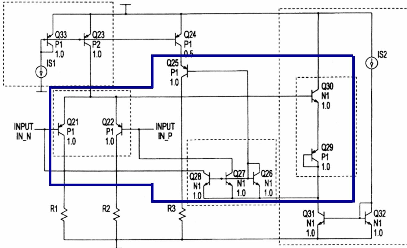
**Q29 & Q30 provide a voltage clamp to track the input bias currents for changes in CM input voltage.**
