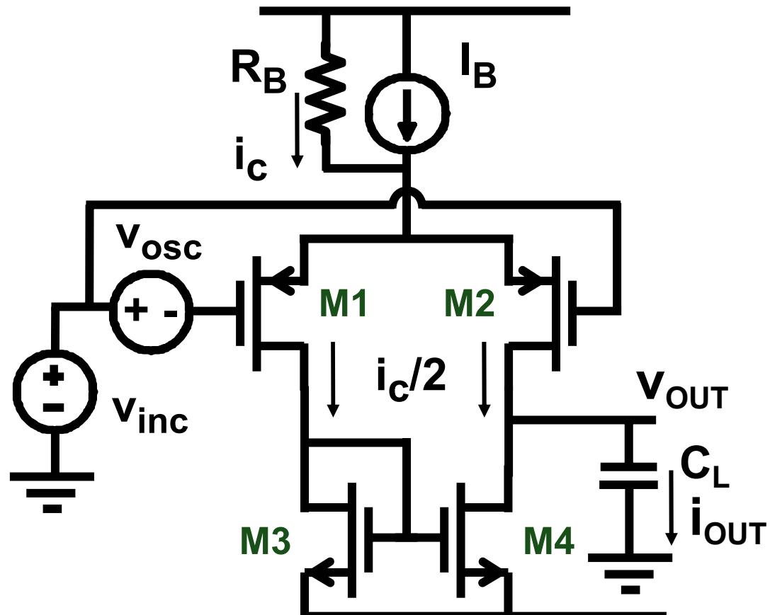
$$\frac{i_{out}}{v_{inc}} = \frac{1}{R_B} \frac{2}{g_m r_o}$$
