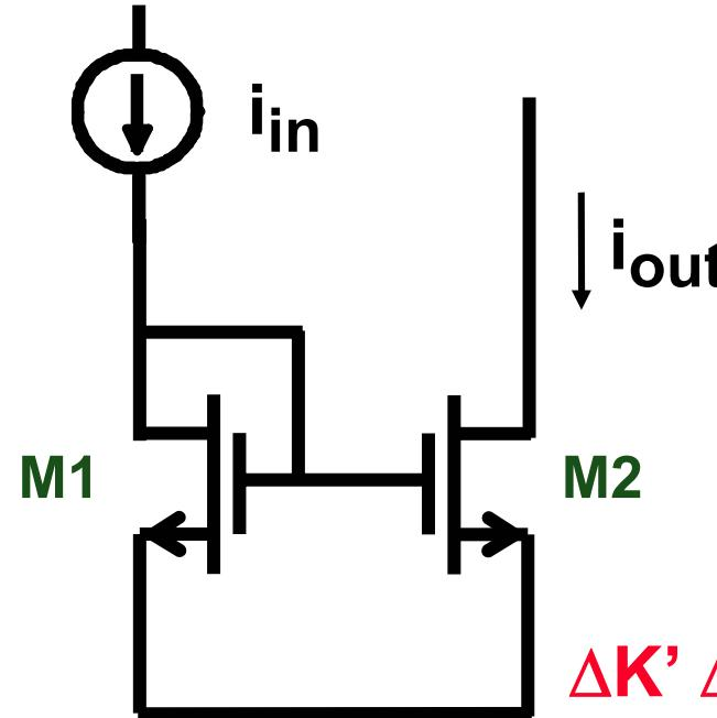
$$\frac{\underline{\Delta I_{out}}}{I_{out}} = \frac{\Delta V_T}{(V_{GS} - V_T)/2} + \frac{\underline{\Delta K'}}{K'} + \frac{\underline{\Delta W/L}}{W/L}$$
