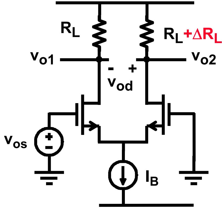
$$v_{od} = \Delta R_L \frac{I_B}{2}$$
