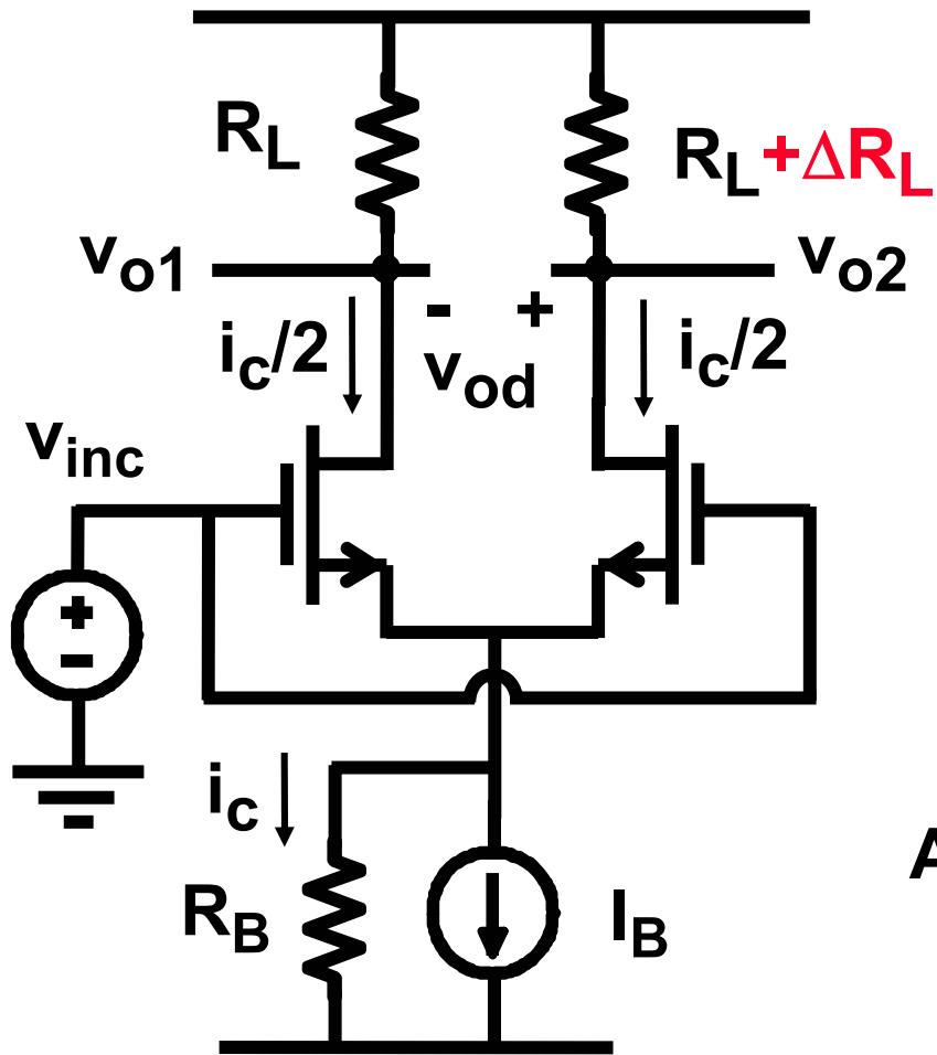
$$A_{dc} = \frac{v_{od}}{v_{ic}} \Big|_{v_{id} = 0} \neq 0$$
