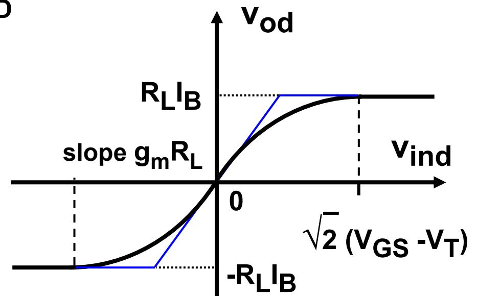
$V_{GS} - V_T$  sets slope
