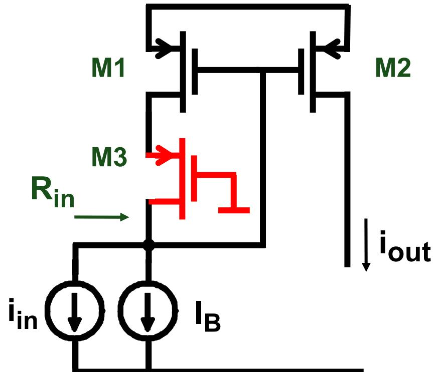
$$i_{out} = I_B + i_{in} \quad R_{in} = \frac{1}{g_{m1}}$$
