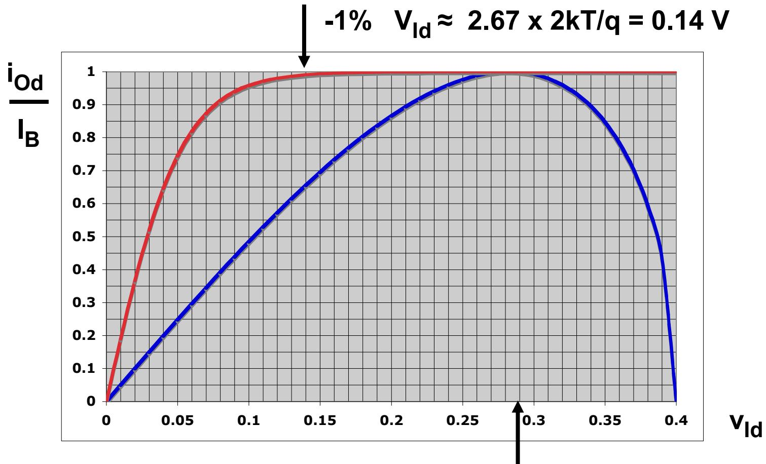
$$V_{Id} = \sqrt{2} (V_{GS} - V_T) = \sqrt{2} \times 0.2 \text{ V}$$
