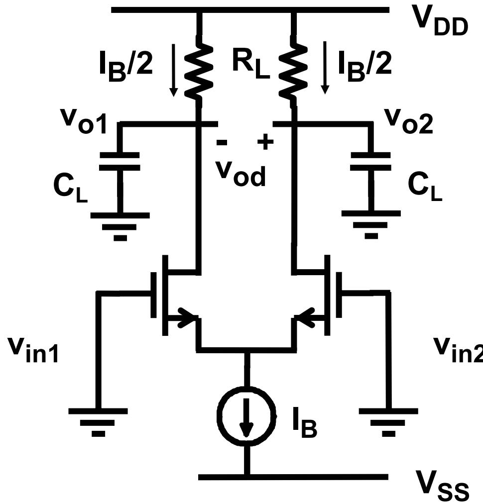
$$v_{in1} = v_{in2} = 0$$
