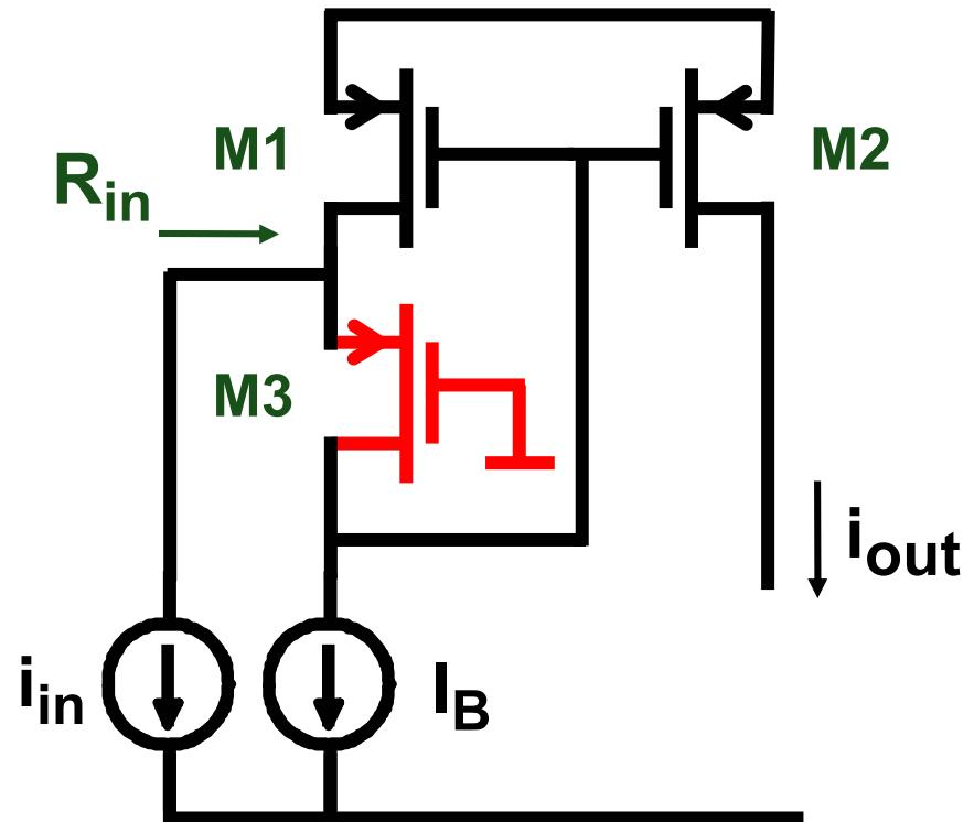
$$R_{in} = \frac{1}{g_{m1}} \frac{1}{g_{m3}r_{o3}}$$
