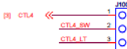
Figure 1-6: CTRL_4 selection jumper
