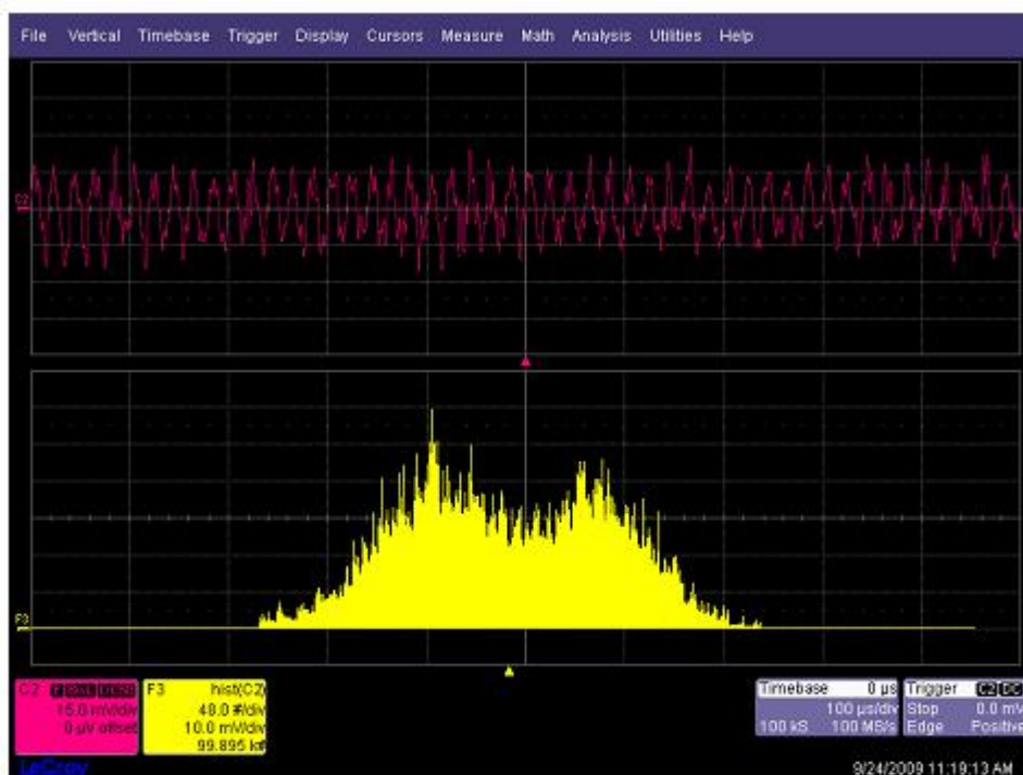
Figure 4: The histogram of a sine contaminated noise source shows two major peaks compared to the single peak in Figure 3
