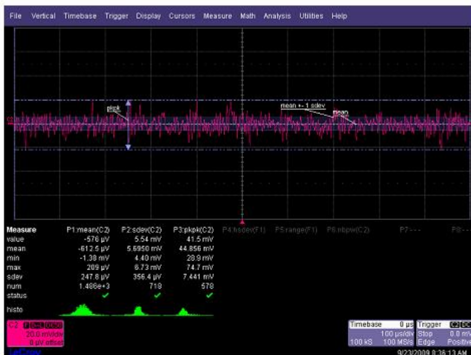
Figure 2: Basic time domain measurement using the mean, standard deviation (RMS), and peak to peak values of a time domain noise waveform
