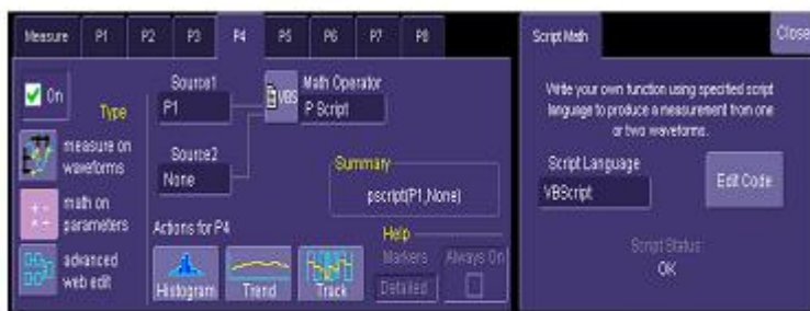
Figure 11: The measurement dialog box for setting up a parameter script to scale parameter P1 to V^2/Hz
