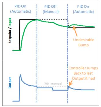
Yikes! The PID jumps back to the last Output value it sent, then starts adjusting from there. This results in an Input bump that we'd rather not have.
