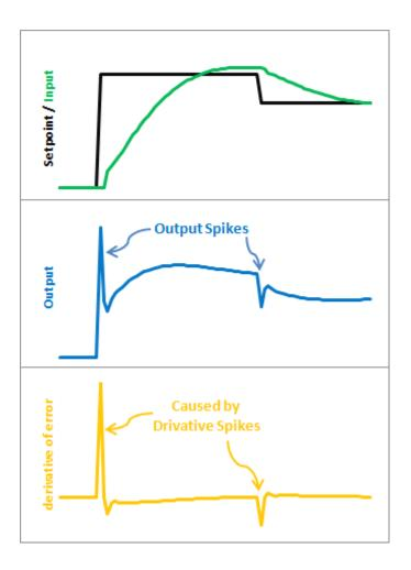
The image above illustrates the problem. Since error=Setpoint-Input, any change in Setpoint causes an instantaneous change in error. The derivative of this change is infinity (in practice, since dt isn't 0 it just winds up being a really big number.) This number gets fed into the pid equation, which results in an undesirable spike in the output. Luckily there is an easy way to get rid of this.
