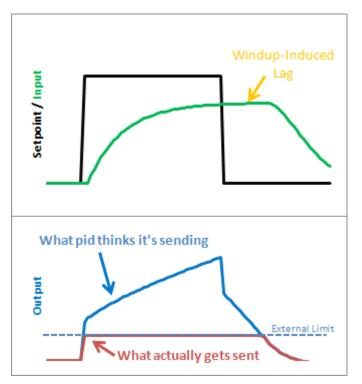
Reset windup is a trap that probably claims more beginners than any other. It occurs when the PID thinks it can do something that it can't. For example, the PWM output on an Arduino accepts values from 0-255. By default the PID doesn't know this. If it thinks that 300-400-500 will work, it's going to try those values expecting to get what it needs. Since in reality the value is clamped at 255 it's just going to keep trying higher and higher numbers without getting anywhere.
