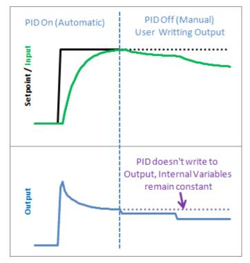
It's true that you could achieve a similar effect by just not calling Compute from the calling routine, but this solution keeps the workings of the PID contained, which is kind of what we need. By keeping things internal we can keep track of which mode were in, and more importantly it let's us know when we change modes. That leads us to the next issue...
