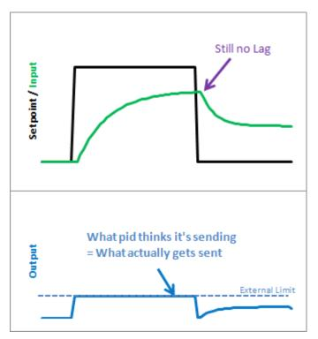
As we can see, windup is eliminated. in addition, the output stays where we want it to. this means there's no need for external clamping of the output. if you want it to range from 23 to 167, you can set those as the Output Limits.
