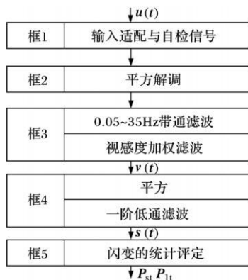
图 1 IEC 推荐的电压波动与闪变测量原理框图 Fig. 1 Diagram of voltage fluctuation and flicker measurement principle recommended by IEC
