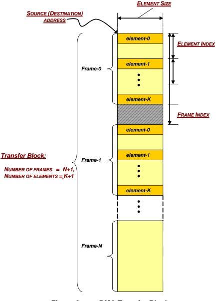
Figure 2. DMA Transfer Block
