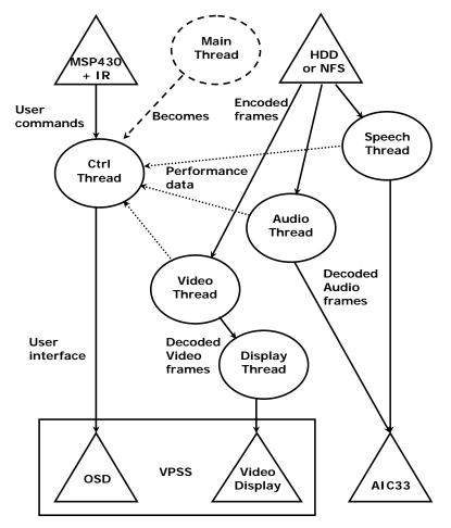
Figure 2. Decode Demo Threads
