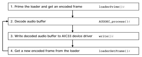
Figure 7. Audio Thread Main Loop Flow
