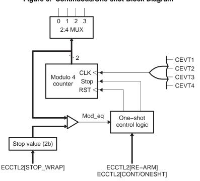
Figure 6. Continuous/One-shot Block Diagram
