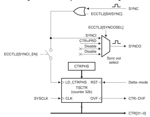
Figure 7. Counter and Synchronization Block Diagram
