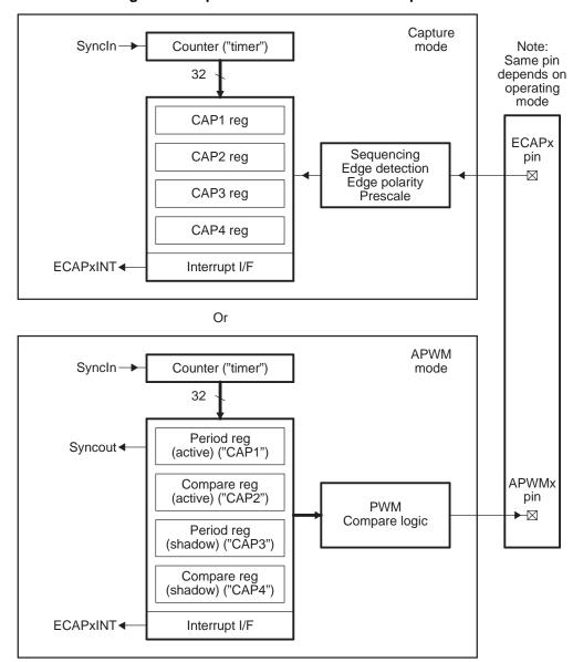
Figure 2. Capture and APWM Modes of Operation
