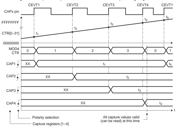
Figure 10. Capture Sequence for Absolute Time-Stamp, Rising Edge Detect
