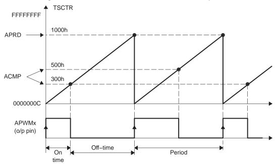
Figure 9. PWM Waveform Details Of APWM Mode Operation
