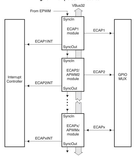
Figure 1. Multiple eCAP Modules
