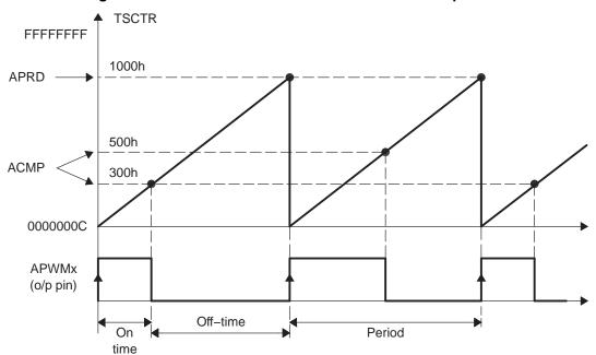
Figure 14. PWM Waveform Details of APWM Mode Operation
