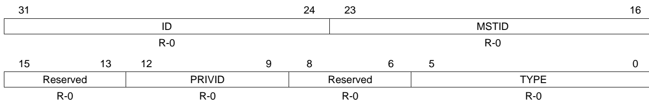
Figure 10-13. Fault Status Register (FLTSTAT)
