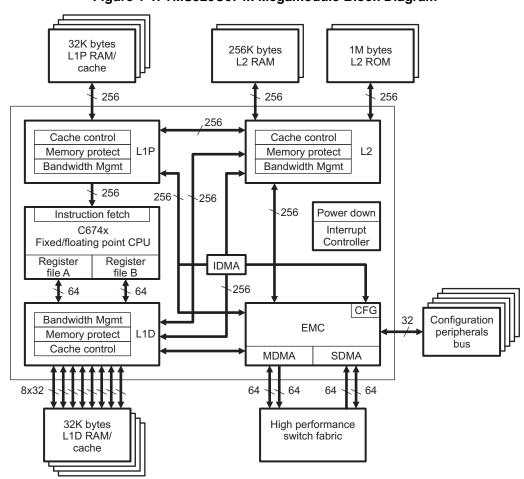
Figure 1-1. TMS320C674x Megamodule Block Diagram
