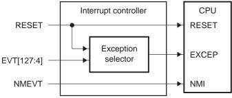
**NOTE:** Reset and NMI are also shown in this diagram. In fact, when exceptions are enabled within the C674x CPU, the NMI signal is used as a non-maskable exception input. These two signals are combined within the CPU along with a variety of other CPU exceptions. For more information on CPU exceptions, refer to the *TMS320C674x DSP CPU and Instruction Set Reference Guide* (SPRUFE8).
