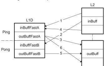
Figure 5-3. Example of IDMA Channel 1
