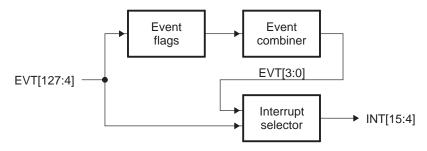
Figure 7-9. CPU Interrupt Routing Diagram
