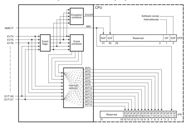
Figure 7-14. CPU Event Routing Diagram
