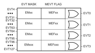
The basic concept of the event combiner is to perform an OR operation on a subset of the system event flags (described in Table 7-2). The results of the OR operation are provided as a new "combined" event).
