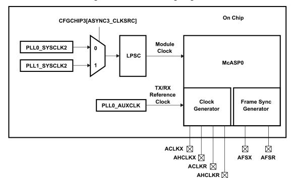
Figure 7-7. McASP Clocking Diagram
