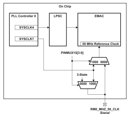
Figure 7-5. EMAC Clocking Diagram
