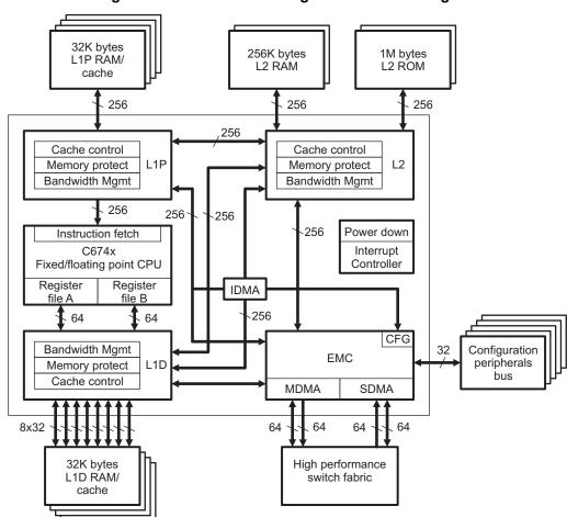
Figure 3-1. TMS320C674x Megamodule Block Diagram
