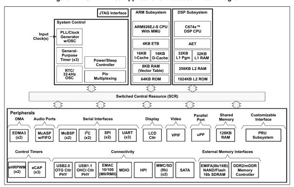
Figure 1-1. OMAP-L138 Applications Processor Block Diagram
