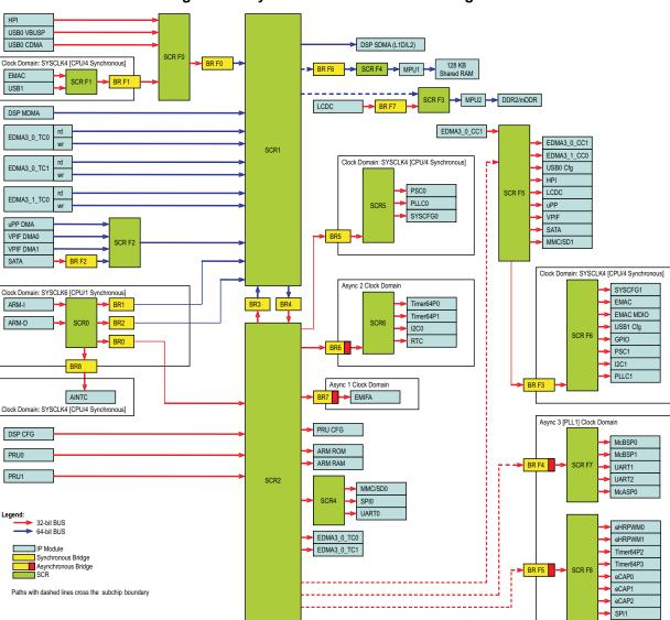
Figure 4-1. System Interconnect Block Diagram
