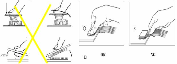
Precaution for soldering the LCM
