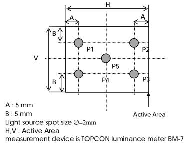
FIG. 5 The definition of viewing angle
