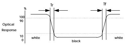
The values specified are at an approximate distance 500 m m from the LCD surface at a viewing angle of  $\Phi$  and  $\theta$  equal to 0°.Measurement condition : Refer to next pages ( B - light source , Halogen Lamp, with polarizer )
