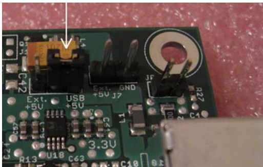
Jumper in USB 5V Position
