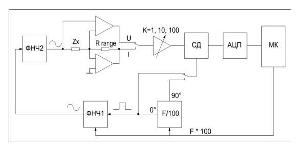
The device used to measure the current active (in the OC) current-voltage converter. Applying the principle of «small fine, a lot», MK manages choice R range and Ku amplifier according to the following table to ensure maximum indication ADC:
