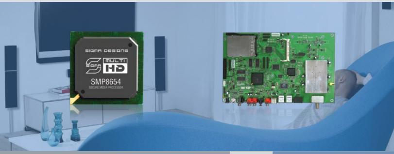
The Tru2way 8654 reference design enables the rapid development of a tru2way<sup>™</sup> DOCSIS 3.0 based cable set-top box or gateway (server for tru2way<sup>™</sup> clients) for cable-TV and IP-Cable systems where downloadable conditional access is used. In addition to enabling a virtually unlimited channel lineup, it supports Voice, Data, Video and Access Control, and can tune to and record up to three TV channels simultaneously.
