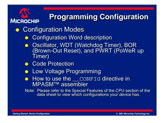
This 14-bit register allows the user to set up the oscillator mode and enable or disable features such as the Watchdog Timer (WDT), Code Protection, and Low Voltage Programming.
