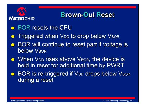
Another feature enabled through the configuration bits is the Brown-Out Reset or BOR. The function of Brown-Out Reset is to reset the CPU when VDD drops below VBOR, this is typically at 4 volts.
