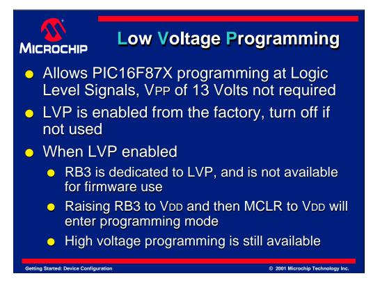
Low Voltage Programming on the PIC16F87X family of microcontrollers can also be enabled through the configuration bits. The Low Voltage Programming feature allows the device to be programmed with logic level signals instead of the traditional 13 Volts on VPP.
