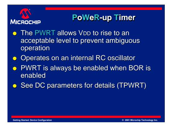
The Power-Up Timer is also enabled through the configuration bits. The Power-Up Timer or PWRT provides a time-out period to allow the VDD to rise to an acceptable level to prevent ambiguous operation.
