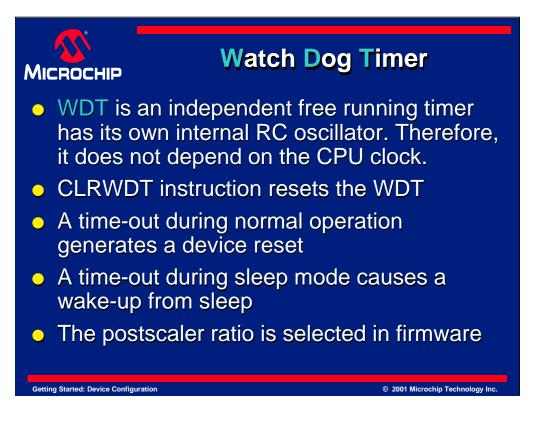
One of the features that is enabled through the configuration bits is the Watchdog Timer or WDT. The Watchdog Timer is an independent free running timer because it has its own onboard internal RC oscillator. This means it does not depend on the CPU clock. Typically the timeout period for the Watchdog Timer is 18ms, but refer to the Electrical Specifications in you device datasheet for specifics and additional information regarding the timeout period for your device.
