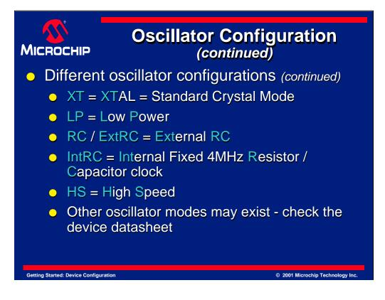
XT represents the Standard Crystal Mode, ranging from 200kHz - 4MHz crystals or 200kHz - 3MHz resonators
