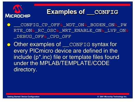
This PIC16F877 example shows the \_\_\_\_CONFIG line defined. The configuration first begins with a space or tab. If a space or tab is not present a warning message will appear stating that the \_\_\_\_CONFIG directive is in column 1.
