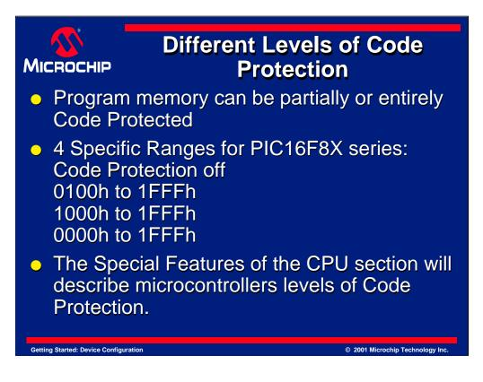
Each microcontroller device has different levels of code protection.
