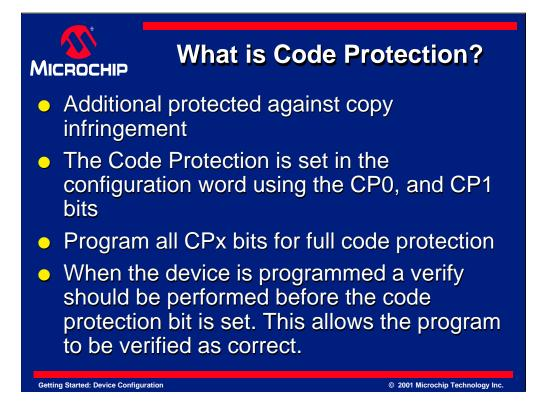
Code Protection is a user selectable feature that provides additional protection for your code and prevents program and data EEPROM from being read out.
