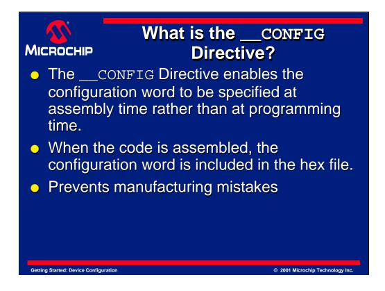
The \_\_\_CONFIG directive enables the configuration word to be present at assembly time rather than at programming time.
