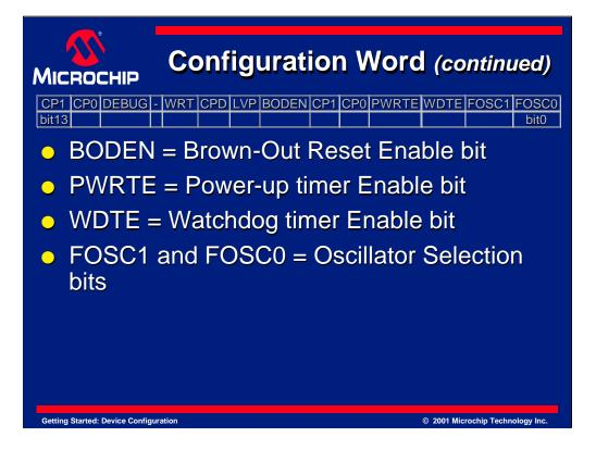
BODEN = Brown-Out Reset Enable bit PWRTE = Power-up timer Enable bit WDTE = Watchdog timer Enable bit FOSC1 and FOSC0 = Oscillator Selection bits
