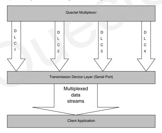
Figure 1: Quectel multiplexer architecture diagram
