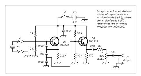
Fig 27.6 — Schematic of the crystal-controlled signal source. All resistors are <sup>1</sup>/<sub>4</sub>-W, 5% carbon units, and all capacitors are disc ceramic. A full-size etching pattern and parts-placement diagram are in Chapter 30, References.
