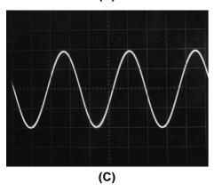
Fig 27.11 — Examples of distorted waveforms. The result of clipping is shown in A. Nonlinear amplification is shown in B. A pure sine wave is shown in C for comparison.
