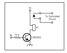
Fig 27.16 — A typical commonemitter switching amplifier.
