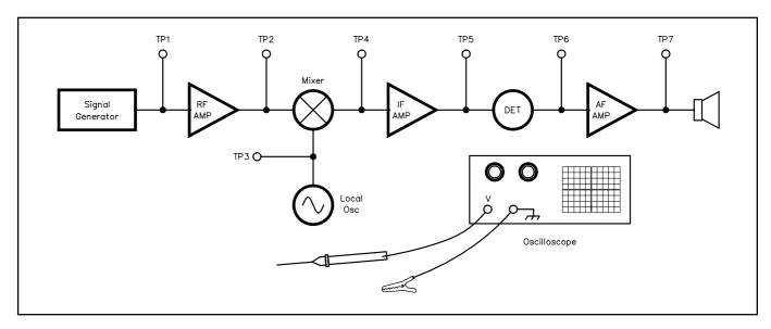
Fig 27.8 — Signal tracing in a simple receiver.
