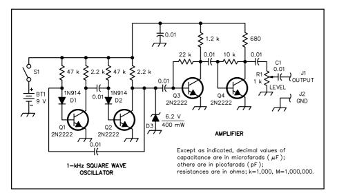
Fig 27.5—Schematic of the AF/RF signal injector. All resistors are <sup>1</sup>/<sub>4</sub>-W, 5% carbon units, and all capacitors are disc ceramic.
