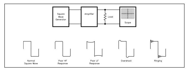
Fig 27.12 — Square-wave distortion and probable causes.
