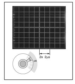
Fig 27.2—An oscilloscope display showing the relationship between time-base setting and graticule lines.
