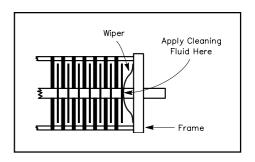
Fig 27.23 — Partial view of an airdielectric variable capacitor. If the capacitor is noisy or erratic in operation, apply electronic cleaning fluid where the wiper contacts the rotor plates.
