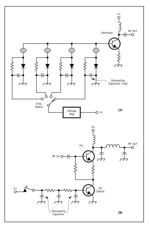
Fig 27.18 — Diode switching selects oscillator crystals at A. A transistor switch is used to key a power amplifier at B.
