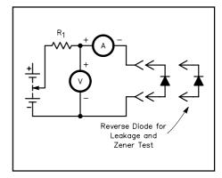
Fig 27.24 — A diode conduction, leakage and Zener-point test fixture. The ammeter should read mA for conduction and Zener point, μA for leakage tests.
