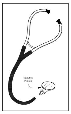
Fig 27.7 — A stethoscope, with the pickup removed, is used to listen for arcing in crowded circuits.
