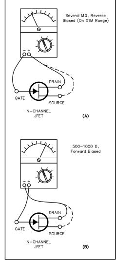
Fig 27.28 — Ohmmeter tests of a JFET. The junction is reverse biased at A and forward biased at B.
