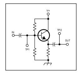
Fig 27.9 — The effect of circuit impedance on an oscilloscope display. Although the circuit functions as a current amplifier, the change in impedance from TP1 to TP2 results in the traces described. This is a common-collector amplifier.
