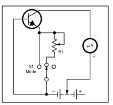
Fig 27.26 — A test circuit for measuring collector-base leakage with the emitter shorted to ground, open or connected to ground through a variable resistance, depending on the setting of S1. See the transistor manufacturer's instructions for test conditions and the setting of R1 (if used). Reverse battery polarity for PNP transistors.
