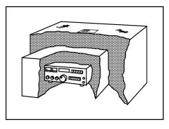
Fig 27.29 — Ship equipment packed securely in a box within a box.
