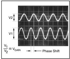
Fig 27.4—A dual-trace oscilloscope display of amplifier input and output waveforms.
