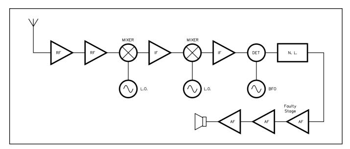
Fig 27.10 — The 14-stage receiver diagnosed by the "divide and conquer" technique.
