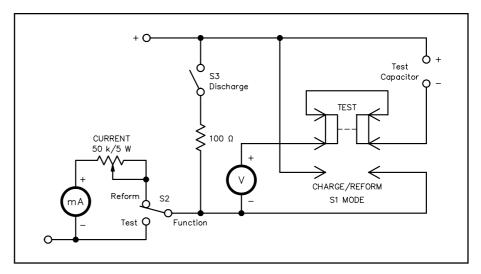
Fig 27.22 — A fixture for testing capacitors and reforming the dielectric of electrolytic capacitors. Use 12 V for testing the capacitor. Use the capacitor working voltage for dielectric reformation.
