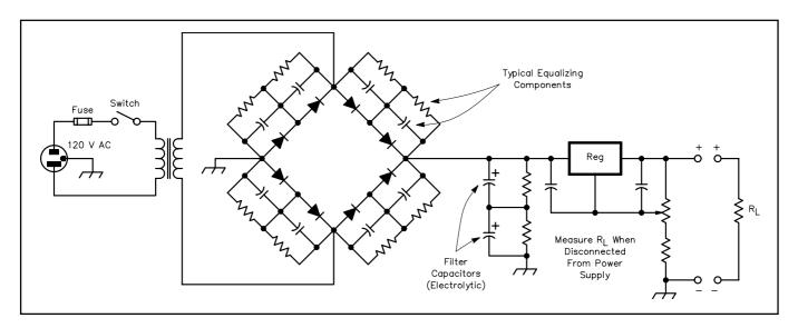
Fig 27.13 — Schematic of a typical power supply showing the components mentioned in the text.
