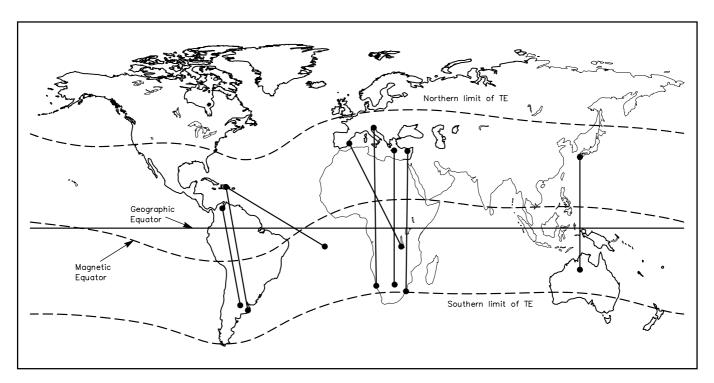
Fig 21.21—Transequatorial spread-F propagation takes place between stations equidistant across the geomagnetic equator. Distances up to 8000 km (5000 mi) are possible on 28 through 432 MHz. Note the geomagnetic equator is considerably south of the geographic equator in the Western Hemisphere.
