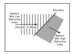
Fig 21.3—Radio waves are refracted as they pass at an angle between dissimilar media. The lines represent the crests of a moving wave front and the distance between them is the wavelength. The direction of the wave changes because one end of the wave slows down before the other as it crosses the boundary between the two media. The wavelength is simultaneously shortened, but the wave frequency (number of crests that pass a certain point in a given unit of time) remains constant.
