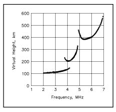
Fig 21.8—Simplified vertical incidence ionogram showing echoes returned from the E, F<sub>1</sub> and F<sub>2</sub> layers. The critical frequencies of each layer (4.1, 4.8 and 6.8 MHz) can be read directly from the ionogram scale.
