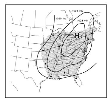
Fig 21.27—Surface weather map for September 13, 1993, shows that the eastern US was dominated by a sprawling high-pressure system. The shaded portion shows the area in which ducting conditions existed on 144 through 1286 MHz and higher.
