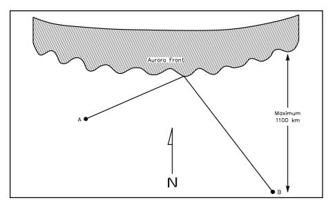
Fig 21.16—Point antennas generally north to make oblique longdistance contacts on 28 through 432 MHz via aurora scattering. Optimal antenna headings may shift considerably to the east or west depending on the location of the aurora.
