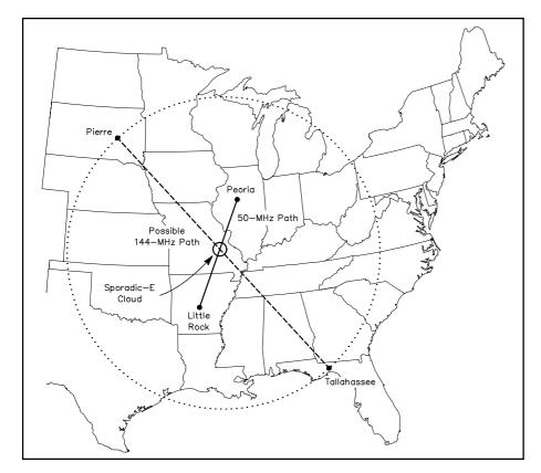
Fig 21.15—50 MHz sporadic-E contacts of 700 km (435 mi) or shorter (such as between Peoria and Little Rock) indicate that the MUF on longer paths is above 144 MHz. Using the same sporadic-E region reflecting point, 144-MHz contacts of 2200 km (1400 mi), such as between Pierre and Tallahassee, should be possible.
