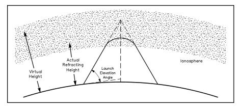
Fig 21.7—Gradual refraction in the ionosphere allows radio signals to be propa-gated long distances. It is often convenient to imagine the process as a reflection with an imaginary reflection point at some virtual height above the actual refracting region. The other figures in this chapter show ray paths as equivalent reflections, but you should keep in mind that the actual process is a gradual refraction.
