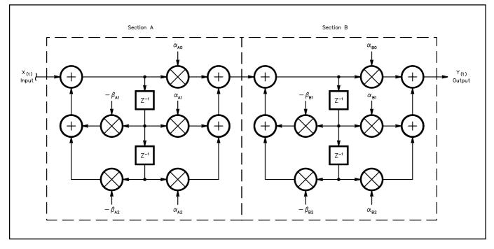
Fig 18.7—Block diagram of a cascade-form IIR filter.
