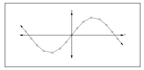
Fig 18.21—Linear piece-wise representation of data resulting from first-order interpolation.
