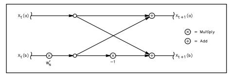
Fig 18.32—Modified butterfly calculation.
