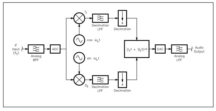
Fig 18.15—Block diagram of a digital AM demodulator.
