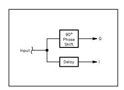
Fig 18.10—Hilbert transformer producing an analytic signal.
