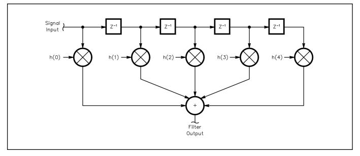
Fig 18.5—Block diagram of an FIR filter for L = 5.
