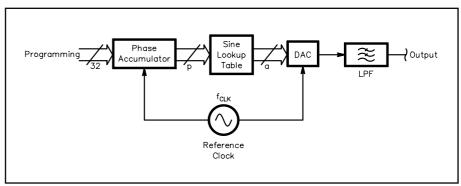
Fig 18.19—DDS block diagram.
