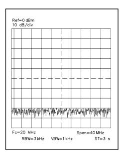
Fig 18.F2—Typical output spectrum of DDS.
