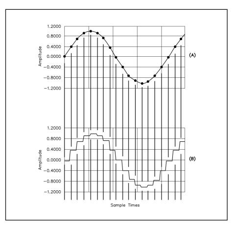
Fig 18.1—Sine wave of frequency much less than the sampling frequency (A). The sampled sine wave (B).
