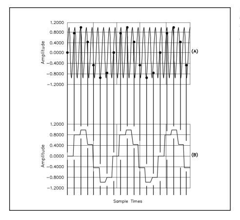
Fig 18.3—Sine wave of frequency greater than the sampling frequency (A). Harmonically sampled sine wave (B).
