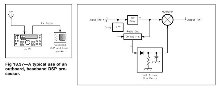
Fig 18.38—Digital AGC system block diagram.
