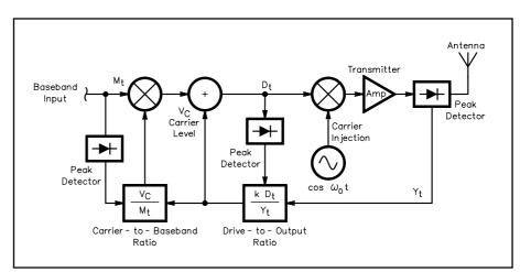
Fig 18.23—AM ALC block diagram.
