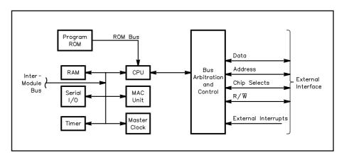
Fig 18.45—Fixed-point DSP block diagram.
