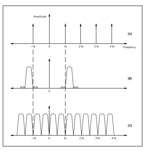
Fig 18.4—Spectrum of sampling impulses (A). Spectrum of a band of real signals (B). Spectrum of a harmonically sampled band of real signals (C). This noise is spread uniformly over the entire input BW of  $f_s/2$ . Taking this and the maximum signal the ADC can handle into account, the maximum signal-to-quantization-noise ratio produced by the ADC is:
