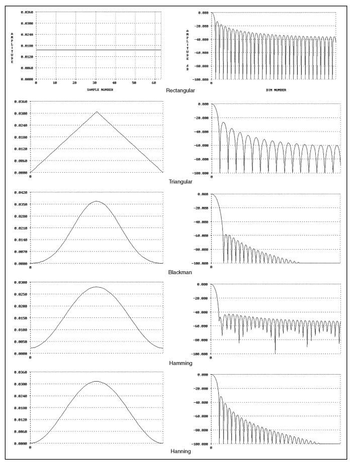
Fig 18.29—Various window functions and their Fourier transforms.
