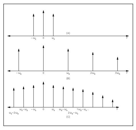
Fig 18.2—Spectrum of an analog sine wave (A). The spectrum of a string of evenly spaced sampling impulses (B). The spectrum of the sampled sine wave (C).
