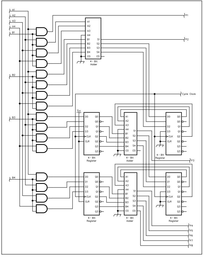
Fig 18.G3—Complete 4-bit multiplier with pipelining.
