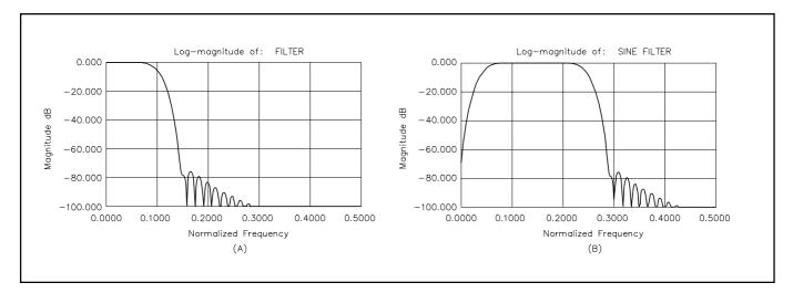
Fig 18.C2—LPF prototype frequency response (A). BPF frequency response of processed impulse response (B).
