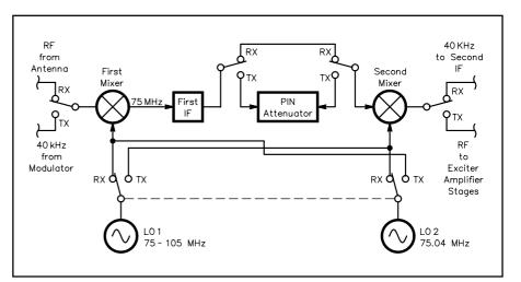
Fig 18.41—Block diagram of IF-DSP conversion scheme with T/R switching added.
