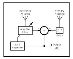
Fig 18.44—Block diagram of a two-antenna, spatial-diversity adaptive system.
