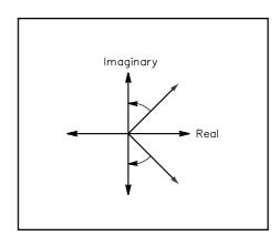
Fig 18.9—Vector representation of a real cosine wave.
