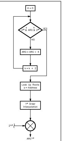
Fig 18.16—Flow chart of a fast square-root algorithm.
