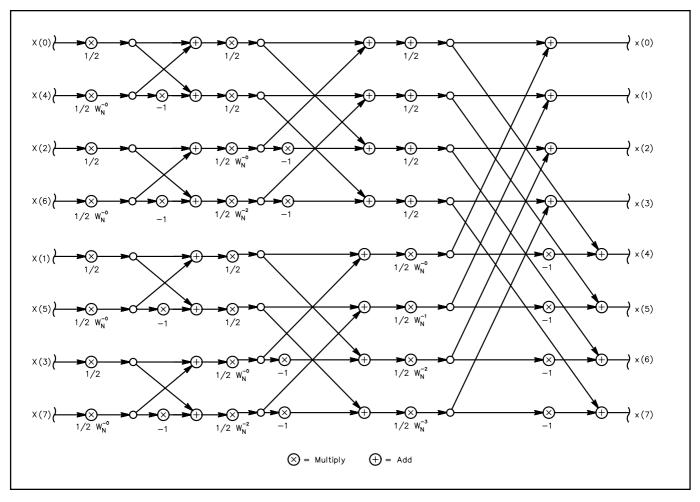
Fig 18.36—FFT<sup>-1</sup> implemented by interchange of inputs, outputs, and coefficients.
