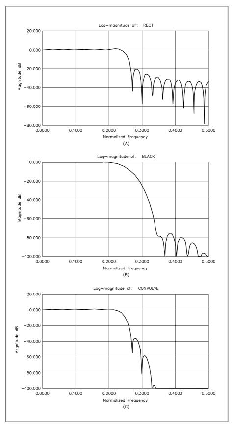
Fig 18.B1—LPF frequency response, rectangular window (A). LPF frequency response, Blackman window (B). LPF frequency response, convolution of filters shown in A and B (C).
