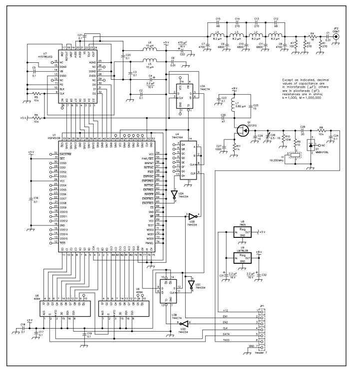
Fig 18.F1—High-performance DDS schematic diagram.
