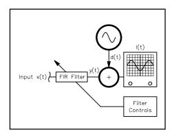
Fig 18.26—An adaptive modeling system, which requires a person at the filter controls.
