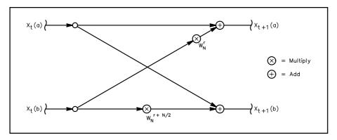
Fig 18.31—Butterfly calculation in a decimation-in-time FFT.
