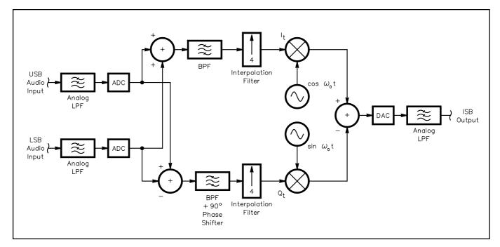
Fig 18.13—Block diagram of a digital ISB modulator.
