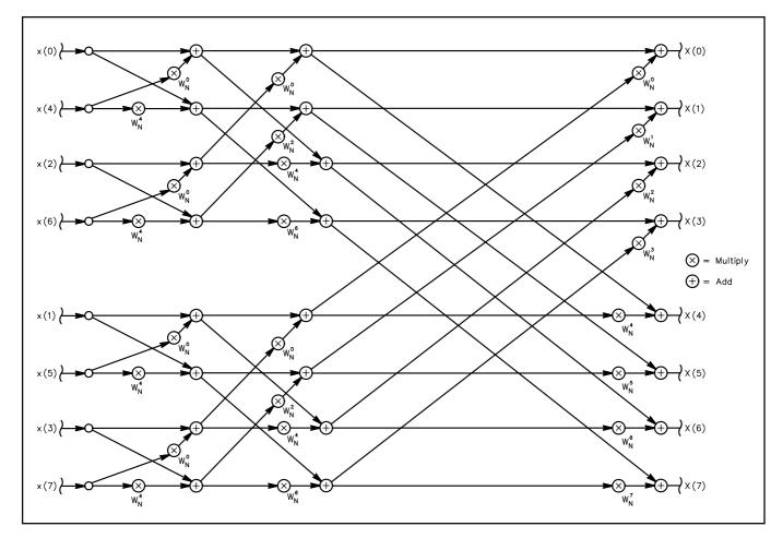
Fig 18.30—Flow chart of an 8-sample FFT.
