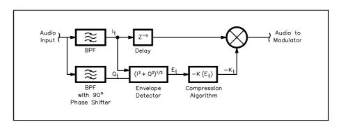
Fig 18.22—Digital RF compressor block diagram.
