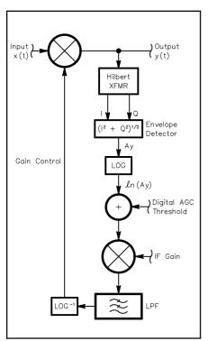
Fig 18.40—IF-DSP receiver with digitally derived analog AGC.
