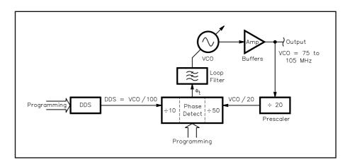
Fig 18.20—Block diagram of a DDS/PLL hybrid synthesizer.
