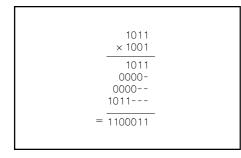
Fig 18.46—Long multiplication of two 4-bit binary numbers.
