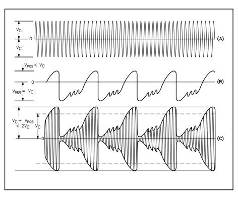
Fig 18.24—AM carrier (A). Baseband input with asymmetrical amplitudes (B). AM modulator output (C).
