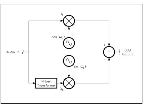
Fig 18.11—Block diagram of a half-complex mixer.
