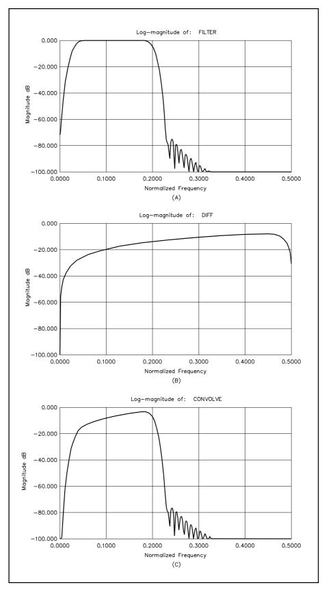
Fig 18.B2—BPF for SSB use, L=99 (A). LPF having rising frequency response, L=31 (B). Frequency response of convolution of filters shown in A and B (C).
