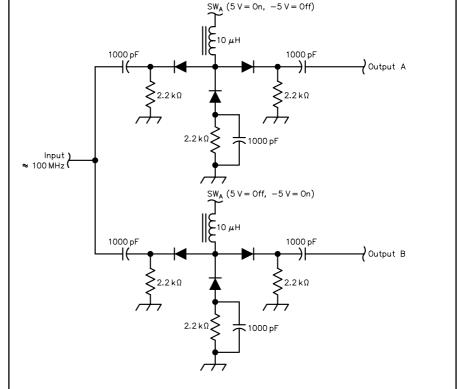
Fig 18.42—SPDT LO switch using PIN diodes. Diodes are Philips BA682 or equiv.
