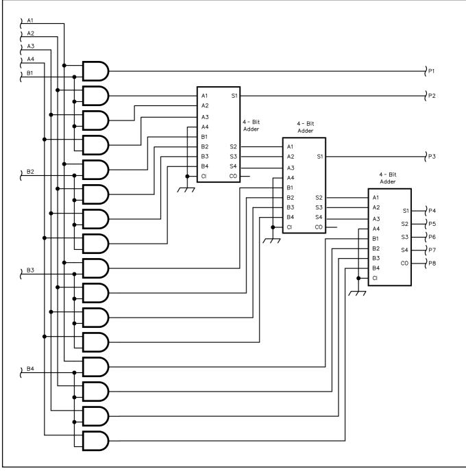
Fig 18.G2—Complete 4-bit multiplier, no pipelining.
