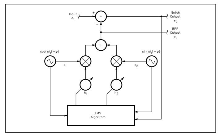
Fig 18.8—Block diagram of a two-tap, adaptive notch filter.
