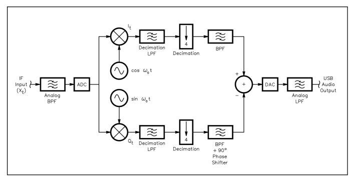
Fig 18.14—Block diagram of a digital SSB demodulator.
