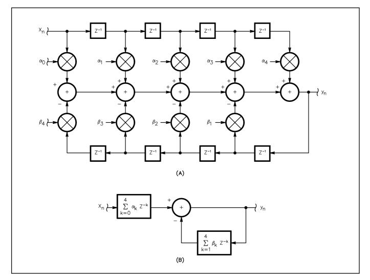
Fig 18.6—Block diagram of an IIR filter for L=5.
