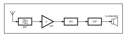
Fig 18.43—DDC receiver block diagram.
