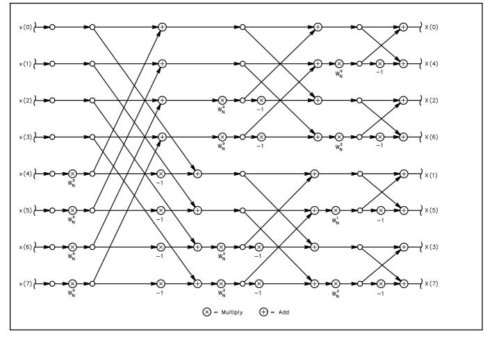
Fig 18.33—Decimation-in-time FFT with different input/output order and modified butterflies.
