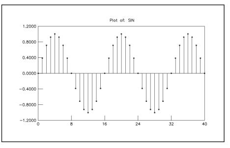
Fig 18.A1—A 40-sample sine wave.
