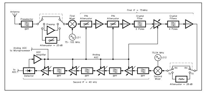
Fig 18.39—IF-DSP receiver block diagram.
