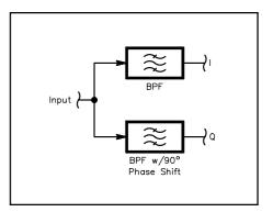
Fig 18.C1—Hilbert transformer using an analytic filter pair.
