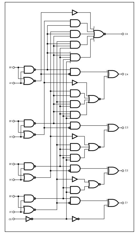
Fig 18.G1—A 4-bit adder schematic diagram.
