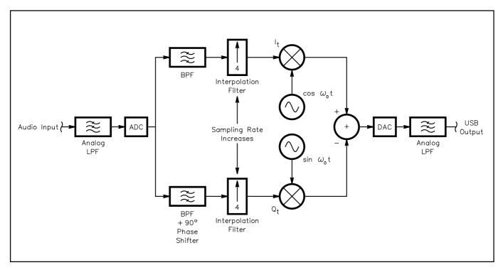
Fig 18.12—Block diagram of a digital SSB modulator.
