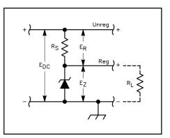
Fig 11.15 — Zener-diode voltage regulation. The voltage from a negative supply may be regulated by reversing the power-supply connections and the diode polarity.
