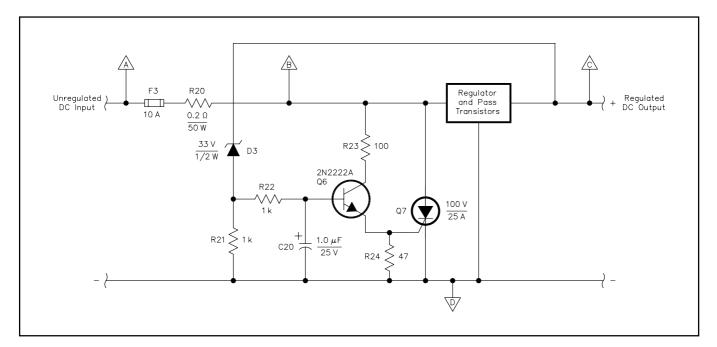
Fig 11.51 — Schematic diagram of the overvoltage protection circuit. Resistors are  $^{1}/_{4}$ -W, 5% carbon types unless noted.
