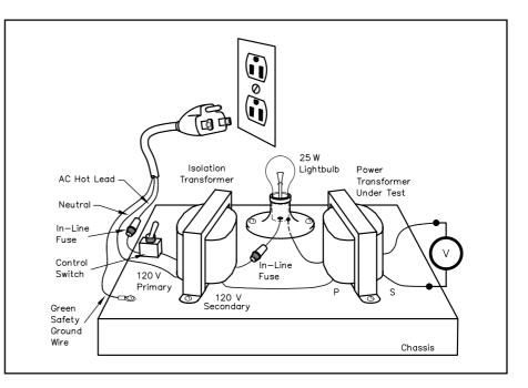
Fig 11.2 — Use a test fixture like this to test unknown transformers. Don't omit the isolation transformer, and be sure to insulate all connections before you plug into the ac mains.
