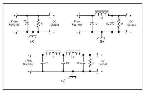
Fig 11.14 — Capacitor-input filter circuits. At A is a simple capacitor filter. B and C are single- and double-section filters, respectively.
