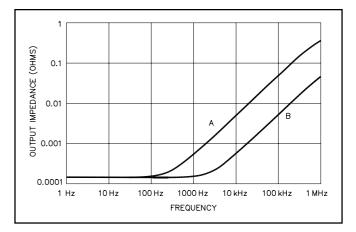
Fig 11.28 — Output impedance magnitude for the voltage-regulator feedback loop.
