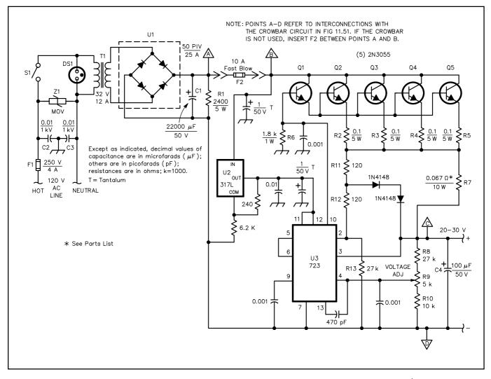
Fig 11.50 — Schematic diagram of the 28-V, high-current power supply. Resistors are 1/4-W, 5% types unless otherwise noted. Capacitors are disc ceramic unless noted; capacitors marked with polarity are electrolytic. Parts numbers given in parentheses that are preceded by the letters RS are Radio Shack catalog numbers.
