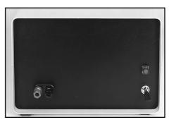
Fig 11.49 — The front panel of the 28-V power supply sports only a power switch, pilot lamp and binding posts for the voltage output. There is room for a voltmeter, should another builder desire one.
