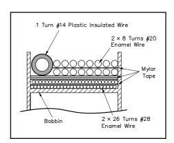
Fig 11.43—Cross-sectional view of T3 (not to scale), showing distribution of windings.
