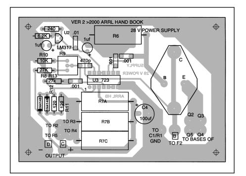
Fig 11.53 — Parts placement diagram for the 28-V power supply. A full-size etching pattern is in the References chapter.
