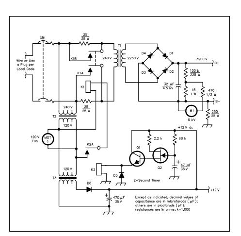
Fig 11.54—Schematic diagram of the high-voltage power supply.
