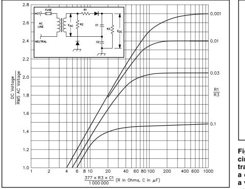
Fig 11.10 — DC output voltages from a full-wave voltage doubler circuit as a function of the filter capacitances and load resistance. For the ratio R1 / R3 and for the R3  $\times$  C1 product, resistance is in ohms and capacitance is in microfarads. Equal resistance values for R1 and R2, and equal capacitance values for C1 and C2 are assumed. These curves are adapted from those published by Otto H. Schade in "Analysis of Rectifier Operation," *Proceedings of the l. R. E.*, July 1943.
