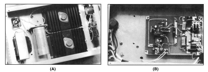
Fig 11.33 — A shows a top view of the open power-supply chassis. The 1/8-in plate holding C1 is visible at the left edge of the heat sinks. B shows a bottom view. Notice that the components are mounted on the etched side of the board. The circuit pattern is simple enough for freehand layout. The front panel is at right in both views.
