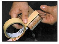
Fig 11.39—Winding the foil tape tightly on the epoxy-coated paper bobbin on the wooden block. The mylar tape is unrolled and positioned over the foil layer as you wind. (*Photo by Dan Wolfgang.*)
