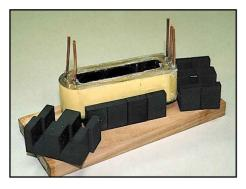
Fig 11.42—Photo showing how the core halves must fit into the completed transformer after it is removed from the wooden block. You will have to file off the rough edges of epoxy to allow the cores to meet properly. The top E-cores have not been inserted into the bobbin yet. (Photo by Larry Wolfgang.)
