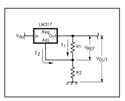
Fig 11.23 — By varying the ratio of R2 to R1 in this simple LM317 schematic diagram, a wide range of output voltages is possible. See text for details.
