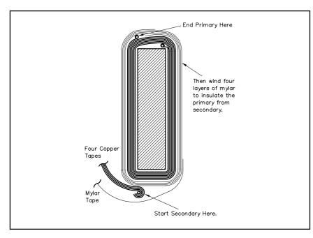
Fig 11.40—Primary 15 turns on bobbin, with start of 4-turn, center-tapped secondary winding.
