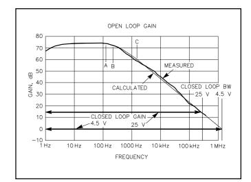
Fig 11.27 — The open-loop frequency response curves of the voltage-regulator feedback loop. Point A is 120 Hz; point B is 280 Hz; point C is 1.2 kHz (above 1.2 kHz, C6 is no longer effective).
