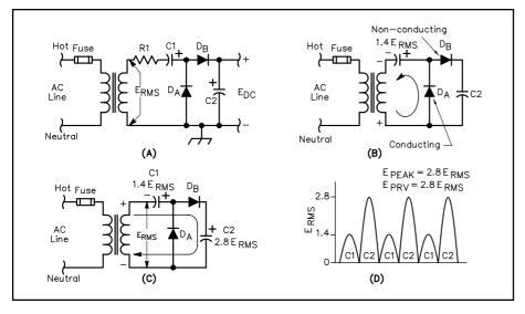
Fig 11.8 — Part A shows a half-wave voltage-doubler circuit. B displays how the first half cycle of input voltage charges C1. During the next half cycle (shown at C), capacitor C2 charges with the transformer secondary voltage plus that voltage stored in C1 from the previous half cycle. The arrows in parts B and C indicate the conventional current. D illustrates the levels to which each capacitor charges over several cycles.
