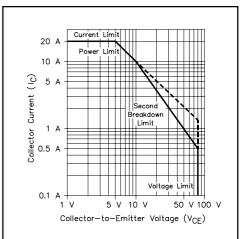
Fig 11.18 — Typical graph of the Safe Operating ARea (SOAR) of a transistor. See text for details. Safe operating conditions for specific devices may be quite different from those shown here.
