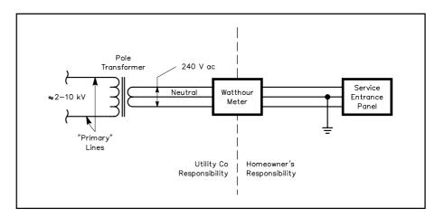
Fig 9.1—Typical division of responsibility for maintenance of electrical power conductors and equipment. The meter is supplied by the utility company.
