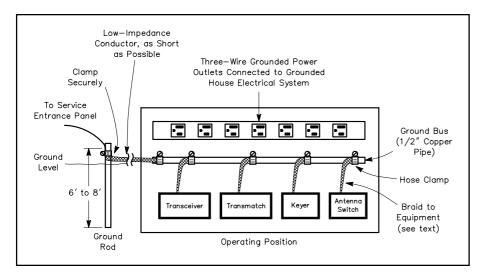
Fig 9.6—An effective station ground bonds the chassis of all equipment together with low-impedance conductors and ties into a good earth ground. Note that the ground bus is in turn bonded to the service entrance panel. This connection should be made by a licensed electrician with #6 AWG (minimum size) copper wire.
