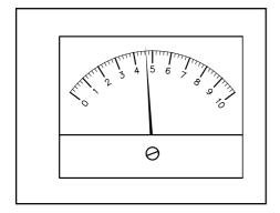
Fig 4.2 — This voltmeter scale reads from 0 to 10 V, with marks every 0.2 V. The meter is reading a value greater than 4.6 but less than 4.7 V. With care you may be able to estimate the reading as 4.68 V, but the digit 8 really only represents a guess. That digit is uncertain because you cannot read it directly from the scale.
