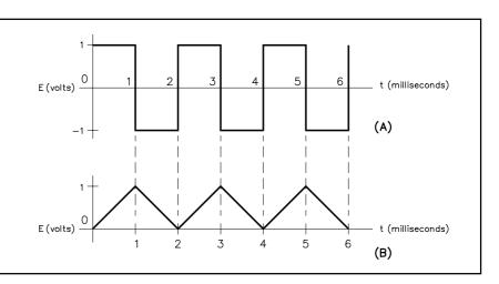
Fig 4.23 — Part A shows a series of square-wave pulses and Part B shows the output from an op-amp integrator with the square-wave input.
