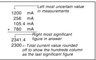
Fig 4.4 — This calculation shows the proper use of the rule for addition and subtraction using significant figures. The current measurements from Fig 4.3 are added to calculate the total circuit current. The resulting value is then rounded off to make the hundreds column the last significant figure.
