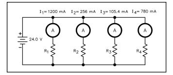
Fig 4.3 — This parallel circuit has four branches connected to the battery. Ammeters measure the current through the branches, with the readings indicated. This circuit illustrates measurements with two, three and four significant figures ( $I_1$  and  $I_4$ ,  $I_2$ ,  $I_3$  respectively).
