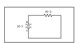
Fig 4.9 — This circuit includes a 20-V battery and a 50- $\Omega$  resistor. The text explains how we can calculate the power dissipated in the resistor.
