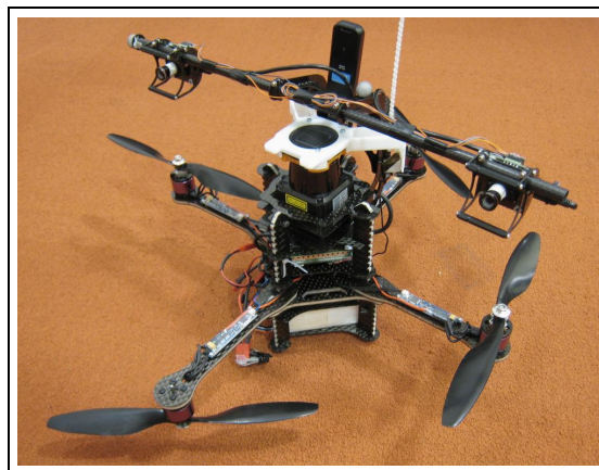
Figure 8. Quadrotor helicopter with Integrated Laser-Stereo Camera
