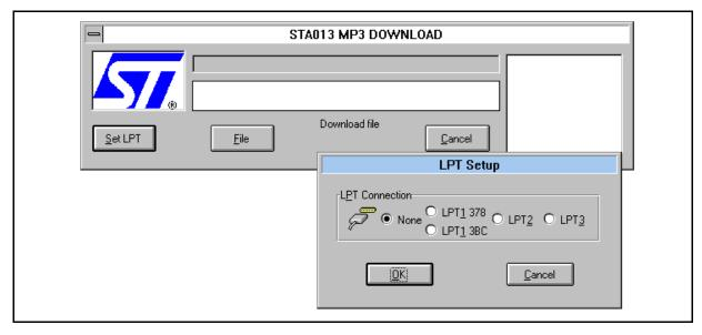
this panel is used to configure the PC Parallel Port address.
