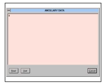
this function allow the user to read the Ancillary Data coded in the MPEG stream. The Ancillary Data are displayed as ASCII characters.
