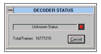
by pressing this button the user open a window displaying the status of STA013. The possible status are described in the STATUS register description.
