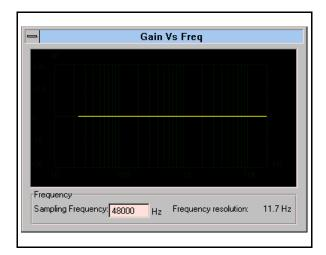
by selecting this function, the user opens a window describing the ideal frequency response of the Tone Control function.
