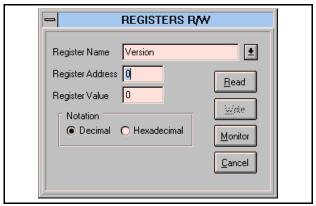
this function allow the read and/or the write operation on all the STA013 registers. To write the registers the user has to update the register setting before pressing the write button.
