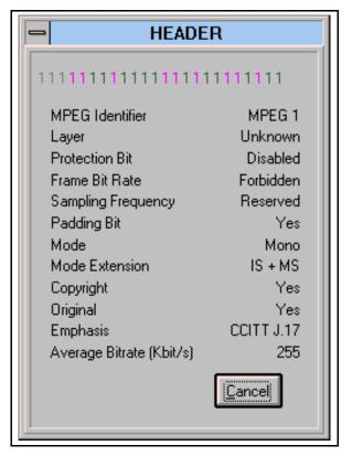
by pressing this button the STA013SDR displays all the relevant information contained in the MPEG Frame Headers of the incoming compressed bitstream.
