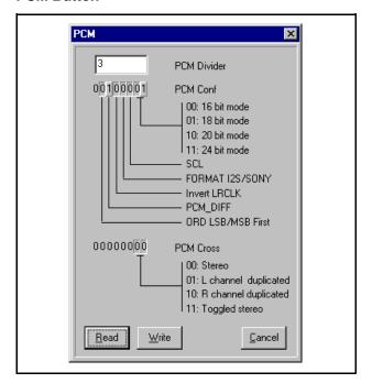
this button, if selected, opens a window to read or change the PCM audio interface configuration.
