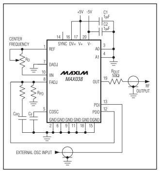
Figure 3. Phase-Locked Loop Using Internal Phase Detector
