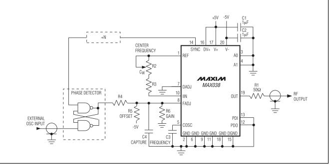
Figure 4. Phase-Locked Loop Using External Phase Detector
