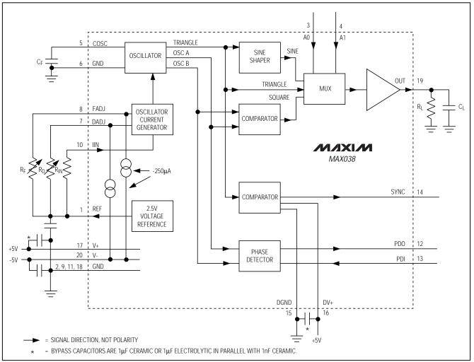
Figure 1. Block Diagram and Basic Operating Circuit
