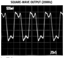
$\begin{array}{l} I_{IN} = 400 \mu A \\ C_F = 20 p F \end{array}$
