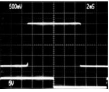
TOP: OUTPUT 50Hz =  $F_{0}$  BOTTOM: SYNC  $I_{IN}$  = 50 $\mu A$   $C_{F}$  = 1 $\mu F$
