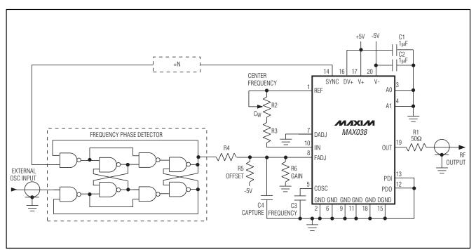
Figure 5. Phase-Locked Loop Using External Frequency Phase Detector
