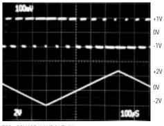
TOP: SQUARE-WAVE OUT,  $2V_{P-P}$  BOTTOM:  $V_{DADJ}$ , -2V to +2.3V
