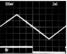
TOP: OUTPUT 50Hz =  $F_0$  BOTTOM: SYNC  $I_{IN}$  = 50 $\mu A$   $C_F$  =  $1 \mu F$
