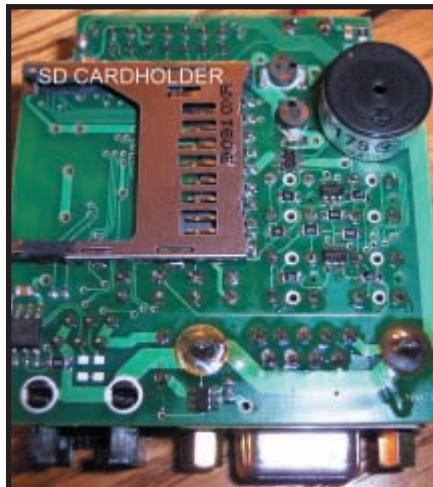
Photo 1 —The board writes files to an SD card, which conveniently allowed us to store many megabytes of data, and then later transfer the data to a computer using readily available hardware. The MSP430 processor can write files to the flash memory card, which subsequently can be opened in Windows Explorer using a standard card reader. It can also read files from the flash memory card stored using a standard card reader/writer.
