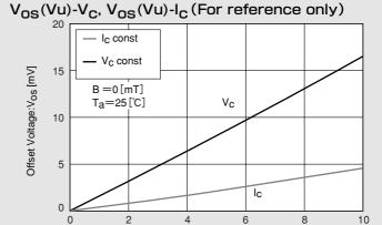
$\begin{array}{l} \text{Input Current:I}_{\mathbb{C}} \ [\text{mA}] \\ \text{Input Voltage:V}_{\mathbb{C}} \ [\text{V}] \end{array}$
