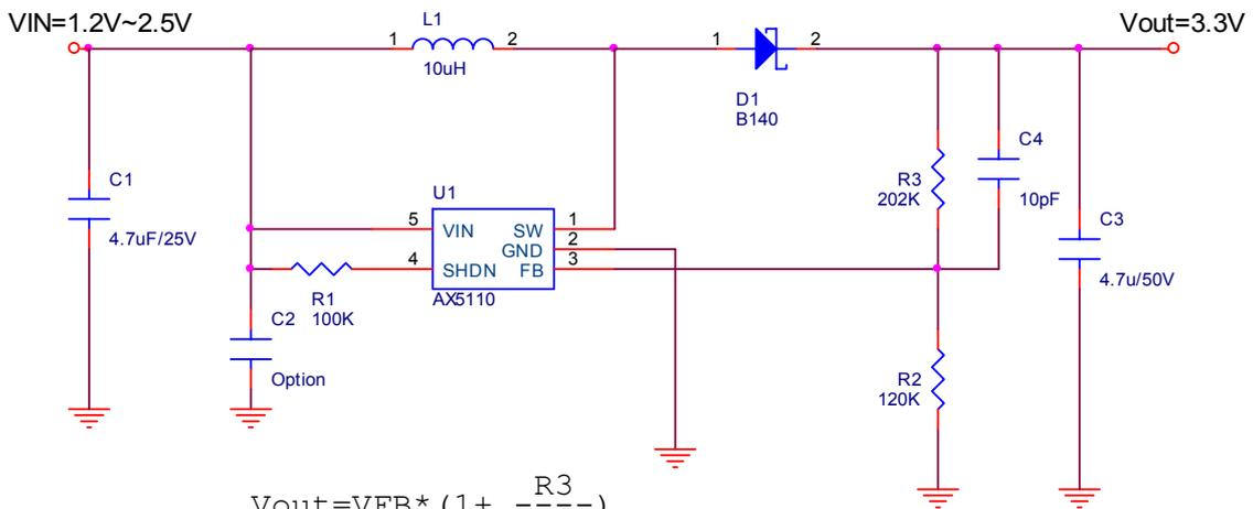
$$V_{out} = V_{FB} * \left(1 + \frac{R_3}{R_2}\right)$$
