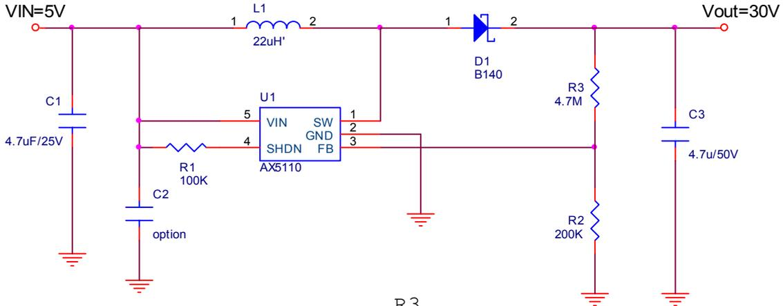
$$V_{out} = V_{FB} * \left(1 + \frac{R_3}{R_2}\right)$$
