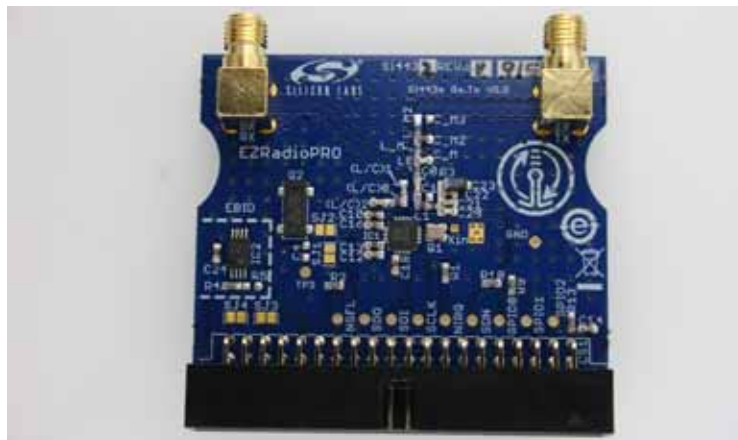
Figure 16. Split TX and RX Testcard (Rx: Left SMA, Tx: Right SMA) for Use with Coaxial Cable and RF Test Equipment for Scientific RF Evaluation
