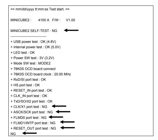
If the test result includes "NG" as shown above, the cause may be a defect in MINICUBE2. Refer to **3.2 Cautions on Self-Testing** and **3.5.2 Action for error**, and retry self-testing. If the same items resulted in "NG" even after the relevant action is implemented, the cause may be a defect in MINICUBE2. In such a case, consult an NEC Electronics sales representative or distributor.
