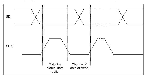
Figure 14: Timing diagram for I<sup>2</sup>C acknowledgement on SDI (SDI=SDA)
