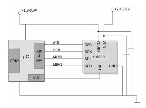
Figure 20: Connection Diagram for use with 3-wire SPI interface
