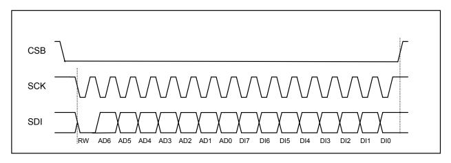
**Figure 10:** For three wire read protocol one extra clock between address byte and data out byte is required. Output data are changed on SDI (SDI=SDA) by SCK rising edge and should be latched by microprocessor during next SCK rising edge.
