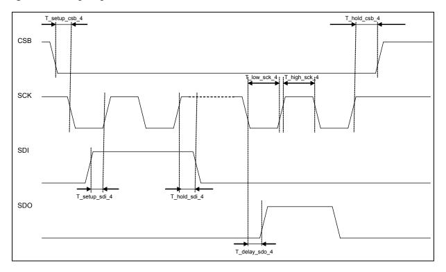
Figure 5: Four wire SPI bit transfer
