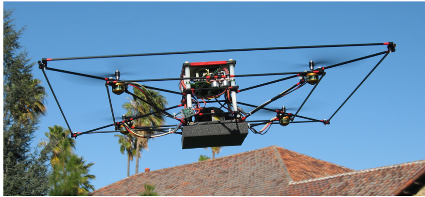
Figure 1. STARMAC II quadrotor aircraft unmanned aerial vehicle (UAV), in flight, with autonomous attitude and altitude control. This is a vehicle of the Stanford Testbed of Autonomous Rotorcraft for Multi-Agent Control (STARMAC) project. Applications include search and rescue, surveillance operation in cluttered environments, and mobile sensor networks. Operation throughout the flight envelope allows characterization of the aerodynamic disturbance effects on the control system, caused by vehicle motion relative to the free stream. The reconfigurable airframe allows the effect of structures near the rotor slip streams to be examined.
