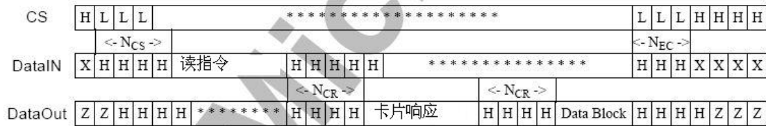
Figure 56: Read CSD - bus timing
