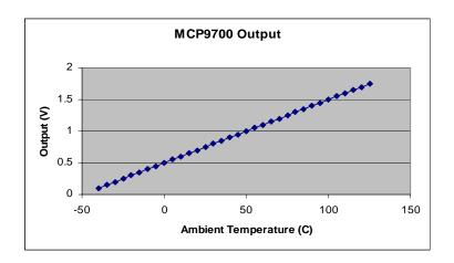
$$V_{OUT} = T_C * T_A + V_{0degC}$$
