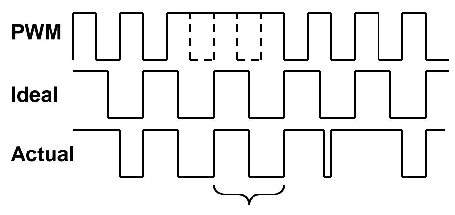
Pulse stretching can be used to obtain a complete period
