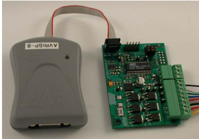
Figure 4-1 . Programming from AVR ISP programmer
