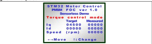
When the motor is running, the LCD indicates the target Id and Iq current components setpoints, as well as the measured values. Pressing the joystick up/down increases (resp. decreases) these settings. Actual speed is also reported.
