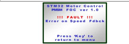
"Press 'Key' to return to menu" is displayed only if the cause of the fault is no longer present. Pressing the 'Key' button causes the main state machine to switch from FAULT to IDLE state. Six different fault sources are monitored during operation. Refer to the UM0492 STM32 sensorless PMSM field-oriented control software library user manual for more implementation details.
