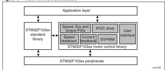
Figure 1. ACIM firmware architecture
