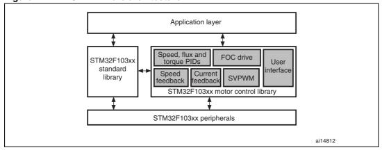
Figure 2. PMSM firmware architecture
